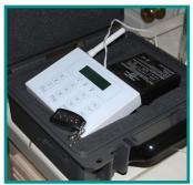
Controller - 110v. or 12v. powered. Receives the message from the wireless sensors, then triggers alarms and/or sends text message to the fumigator.
