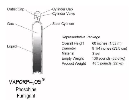
The product flows to the blending equipment through the cylinder outlet valve. As gas is withdrawn from the cylinder, some of the product vaporizes to fill the remaining space in the cylinder. Through this vaporization, the cylinder pressure is maintained.
