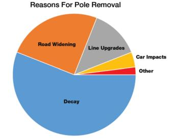
**Figure 2** - While decay was the chief reason for removing a wood pole, the number of poles removed for road widening and line upgrades comprised nearly 38 percent of removals according to a survey of utilities. These poles could be candidates for reuse, which should be factored in when determining the overall service life. (Source: 2007 OSU Utility Pole Research Cooperative Annual Report)
